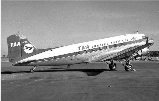
*VH-SBM at Adelaide during the evaluation test phase (Note the paint removed from the top of the fin for the transmitter antenna and the receiver's whip antenna fitted in the ventral position.) Image kindly provided by Geoff Goodall (<https://www.goodall.com.au/default.htm>)*
