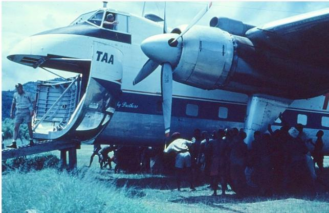
*Pushing the aircraft up to the ramp to unload motor vehicles.*
