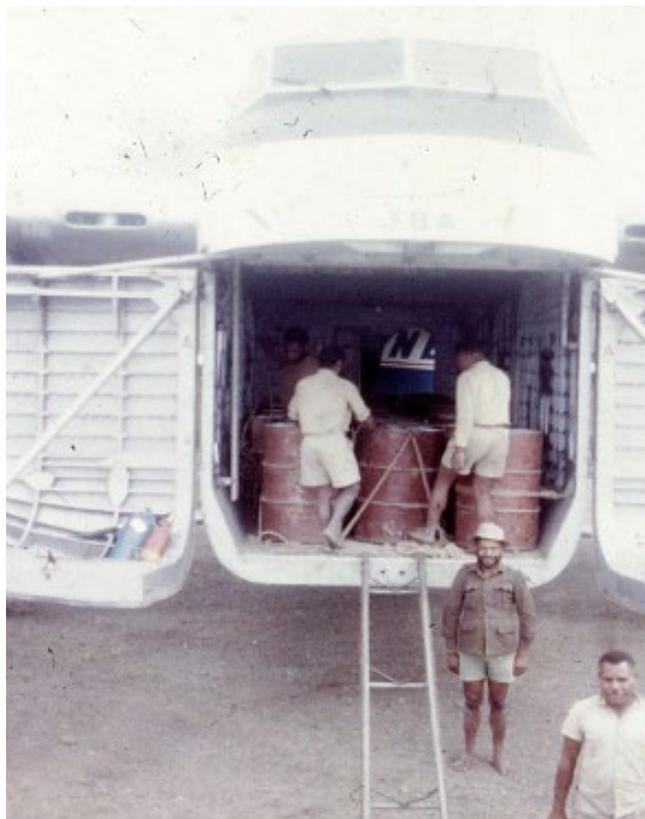
*A typical Bristol fuel cargo load showing just 3 of 26 drums of aviation fuel within the cargo bay, merely tied to the plywood floor with rope. Earthing wires were clipped to each drum and then connected to the fuselage structure to minimize the risk of static electricity fires. Note the two fire extinguishers (on the door), optimistically provided to put out a potential fire of 1100 gallons of fuel!*
