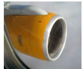
Over half the RB211-535E4s in Icelandair's fleet have exceeded 15,000 hours before removal
