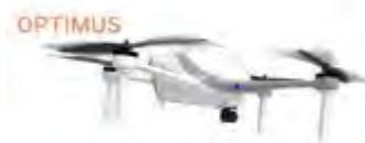
The Airobotics drone lifts off from an air base – which looks like a giant photocopier – and removes humans from such reporting jobs. The drone flies to its assigned position before returning to base after about 33 minutes. (It will soon be able to fly for 44 minutes and even longer as battery quality continues to improve.)
