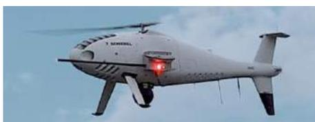
CAMCOPTER® S-100 performed two successful flights of about four hours during the trial and provided compliant measurements of sulphur emissions. The certified sniffer provides live readings of the sulphur level in the ship's exhaust plume. In addition to the sulphur sniffer and the AIS, the CAMCOPTER® S-100 was equipped with an L3 Harris Wescam MX-10 real-time Electro-Optical/Infra-Red (EO/IR) camera.
