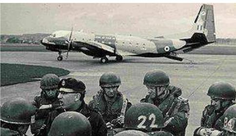
a short-range tactical transport aircraft. In order to produce the required thrust, it was refitted with larger RR Dart engines and propeller blades (14 feet disc). The longer blades required a longer undercarriage, which meant it was extremely hard to load and unload the aircraft. The answer was to enable the aircraft to kneel! Our party trick was to do a high approach and short field landing (selecting
