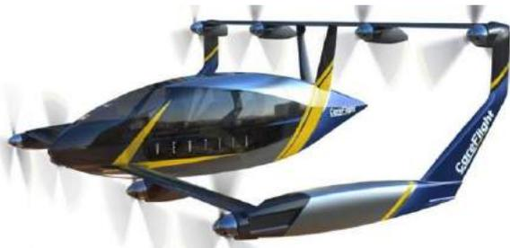
Vertiiia is an electric vertical take-off and landing (eVTOL) aircraft, designed to cruise at a speed of 300kph, and travel up to 250km on electric power or 800km if powered by hydrogen. The partnership could see CareFlight deploy electric flying air ambulances within a few years, which will initially be flown by CareFlight pilots. CareFlight is also providing expert advice and input into the aircraft design to ensure it is fit for medical purposes.
